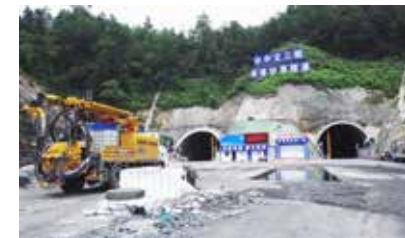
HPC30V混凝土喷浆车 贵州荔榕高速姑两隧道 HPC30V truck-mounted concrete spraying machine Guliang tunnel along Lirong expressway in Guizhou
