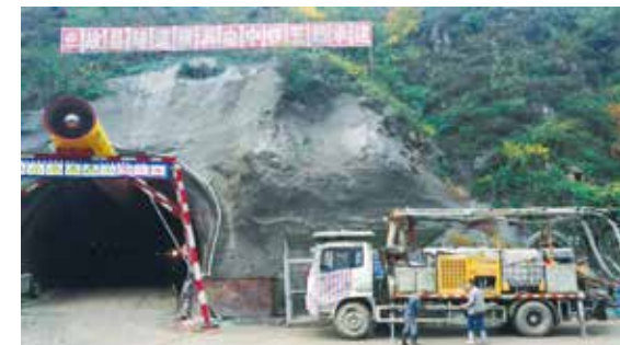
HPC30V混凝土喷浆车 河南洛阳故县隧道 HPC30V truck-mounted concrete spraying machine Guxian tunnel in Luoyang, Henan
