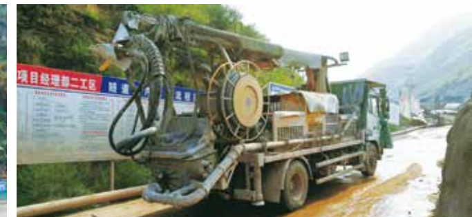
HPC30V混凝土喷浆车 陕西韩城集义隧道 HPC30V truck-mounted concrete spraying machine Jiyi tunnel in Hancheng, Shaanxi
