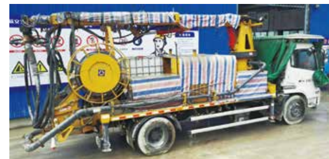
HPC30V混凝土喷浆车 浙江台州合溪里隧道 HPC30V truck-mounted concrete spraying machine Hexili tunnel in Taizhou, Zhejiang
